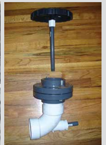
Made with off-the-shelf slip flanges, the only modification is to grind the ridges down flat so the whole flange seals to the liner. We like 5/8" x 3" stainless bolts epoxied into the bottom flange for 4"-8" drains.
