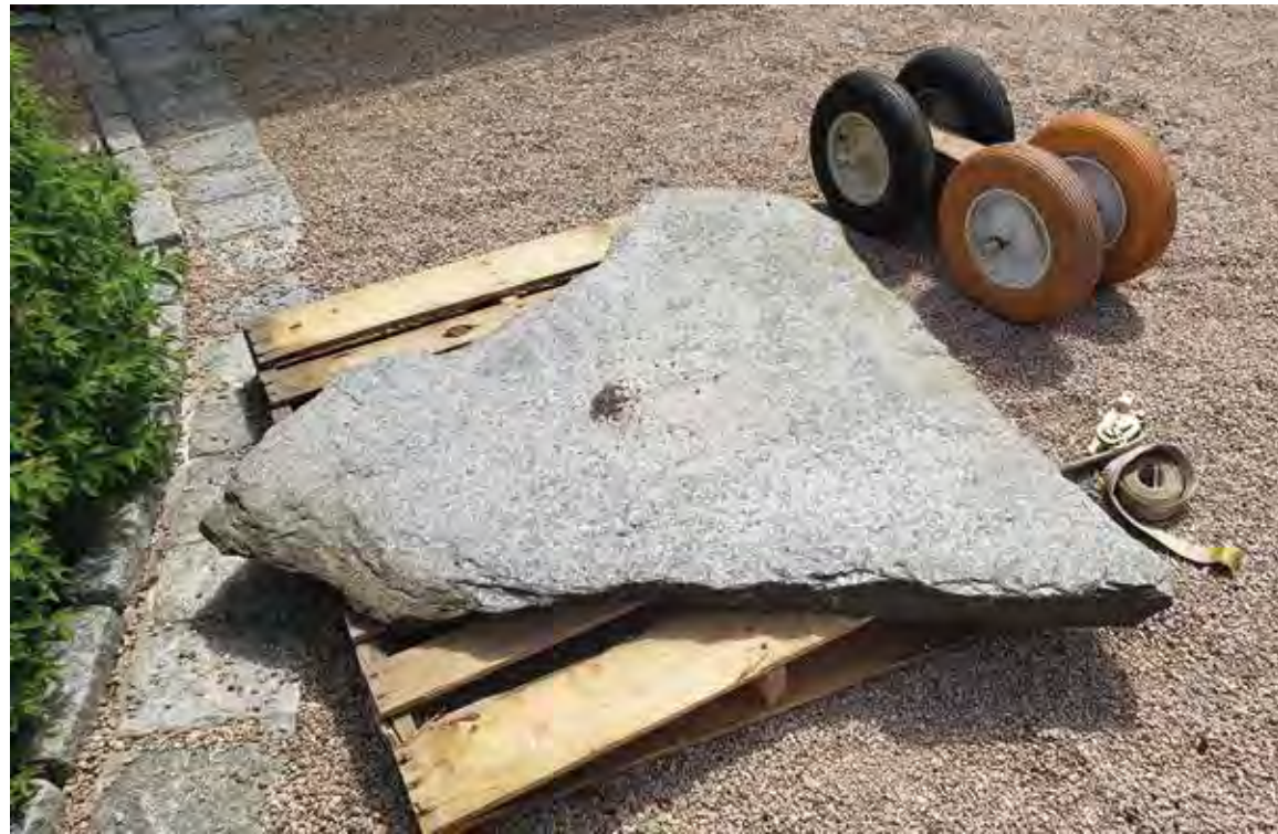
We made this simple dolly with two solid and two pneumatic wheelbarrow tires. We found rolling the slab with solid tires in front made for easier steering.
