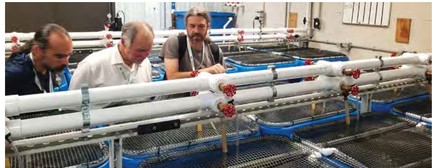
Researchers from universities in New Mexico and Canada inspect the recirculating aquaculture research system at Kentucky State.
