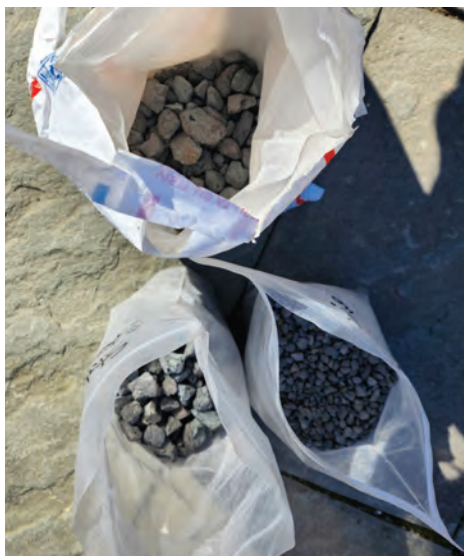
Our tri-blend of ceramic, structural and lightweight aggregate (left) was implemented into our "sun shelf" wetland filter (above).
