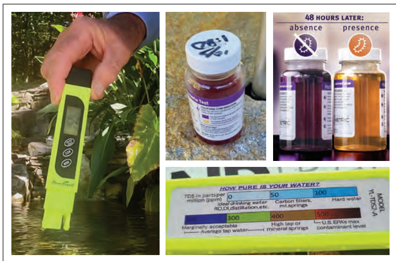
Testing equipment (left inset) should include total coliform count, E. coli tester and total dissolved solids meter. A main wetland filter (above) is constructed within the stream area.
