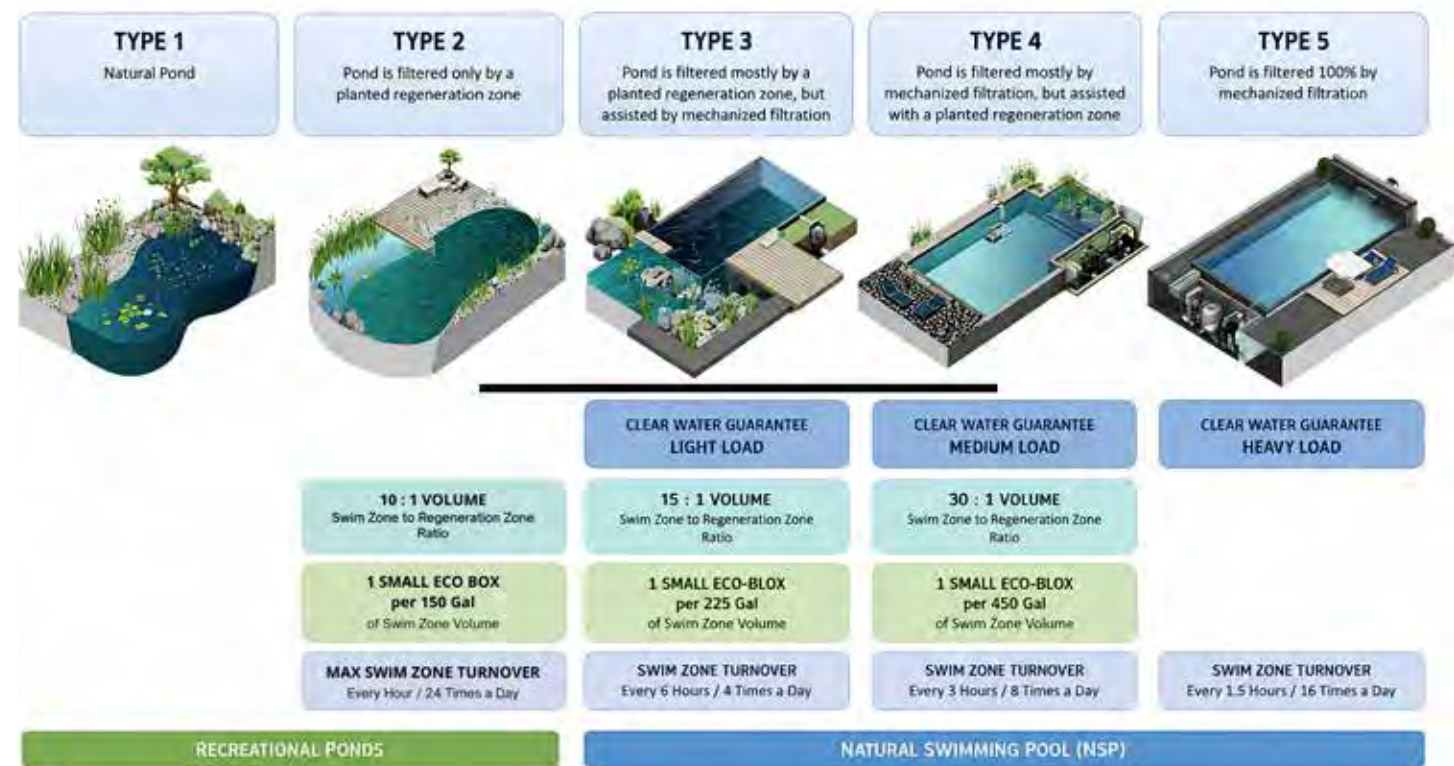
Diagram 2: The five recreational pond and natural swimming pond classifications differ in their use of biological and mechanical filtration. As systems progress from Type 1 to Type 5, water clarity increases while regeneration zone requirements decrease.
